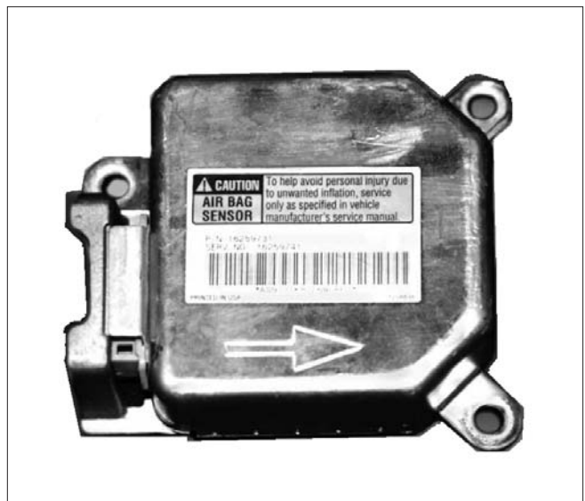
Figure 2: The General Motors Airbag or Sensing and Diagnostic Module (SDM) is an Event Data Recorder (EDR) found in GM passenger vehicles.
